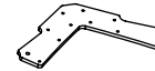
Item 6 Roof Joint Piece X 2 (Note:- extra holes used in manufacture not required for assembly)
